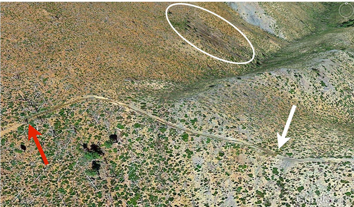
Figure 6 - Google Earth scene of a portion of Cleopatra Ridge and shallow groundwater flow interrupted by McGrew Trail. The water emerges near the red arrow, pools on the surface, and then flows down McGrew Trail for about 700 feet, before dispersing in the area of the white arrow. The white oval is likely a hill slope Darlingtonia wetland above Taylor Creek, although smaller than the ones in Figure 5.
