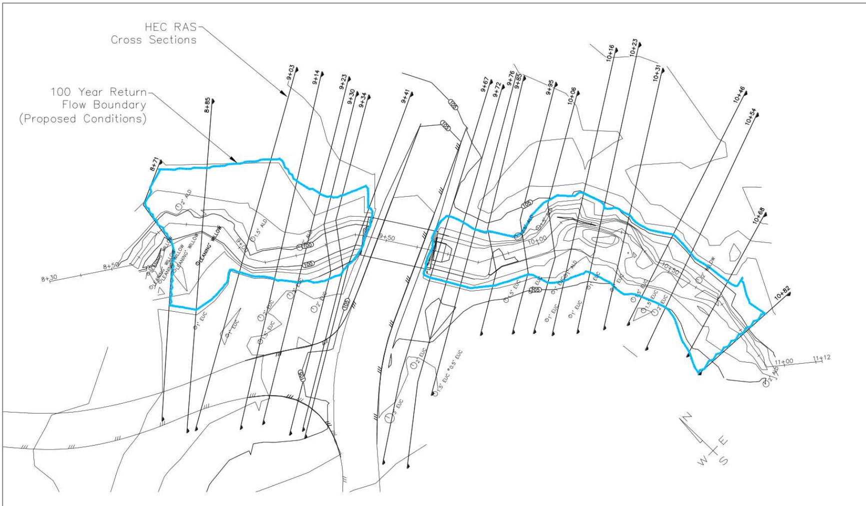
HEC RAS Model domain for South Fork Rawson Creek, Crossing No. 3. Aluminum Box Culvert embedded 3 feet.
